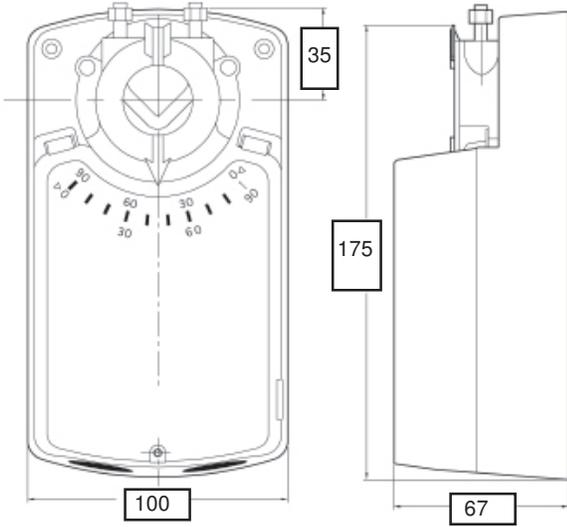
Max size for round shaft is 20 mm in diameter.
