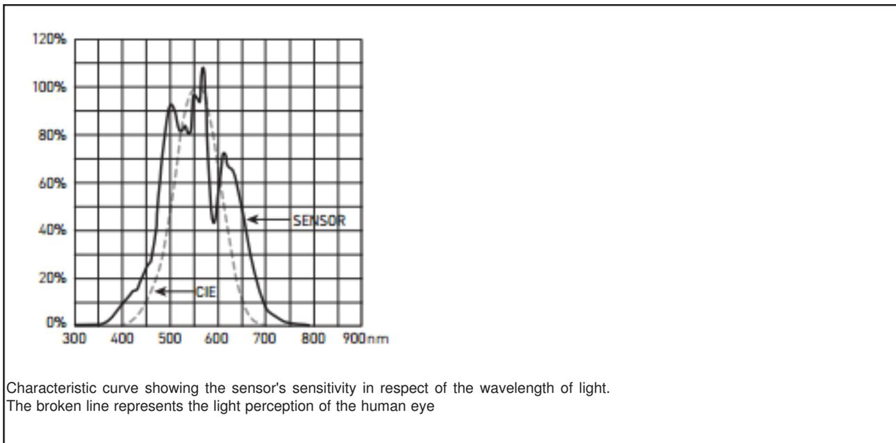
The sensor used in light intensity transmitter LLR was specifically adapted to the sensitivity of the human eye. Its greatest sensitivity is in the range of 350 nm to 820 nm. Therefore with its special filter the sensor is predestined for exposure measurement of daylight and / or for measuring artificial light of high colour temperature (similar to sunlight).
